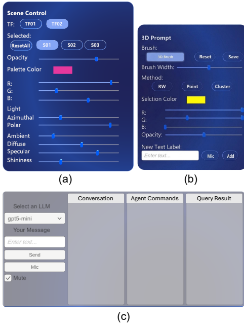
Fig. 1: User interface of Super-Gaussian in the VR environment. (a) Scene control panel for GUI-based Scene editing. (b) 3D prompt panel for brush interaction, selection control, and semantic labeling. (c) NLI interface for voice-command-based volume exploration and scene editing.
